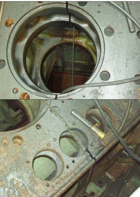
Fig 4 A cutting pattern was devised to meet the least resistance, e.g. cutting through voids within the block
