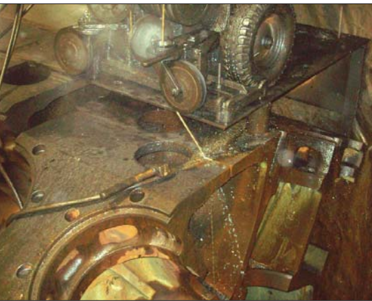
Fig 2 An electroplated diamond wire used because of its qualities in cutting metallic objects
