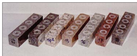
Fig 5 Array of specimens: grooves cut by diamond bit are clearly visible
